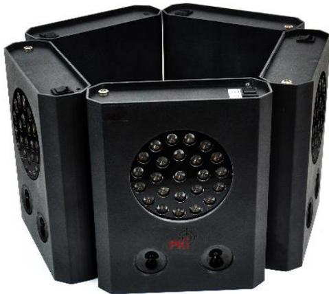
If larger beam angles are required, 3-5 units of **PKI 6715** can be combined to achieve the desired success. For larger conference rooms, a **PKI 6715** 5 pack Audio Jammer can be assembled to provide 360° omnidirectional coverage. Individual installation in conference rooms is of course also possible. With our ultrasonic detector PKI 6705 you can optimize the position of the devices to achieve the perfect coverage.
